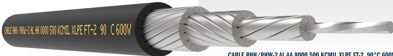
CABLE RHH/RHW-2 AL AA 8000 500 KCMIL XLPE FT-2 90°C 600V
