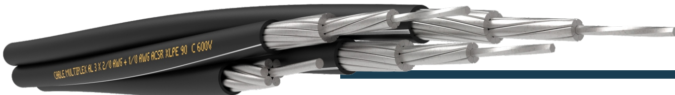
CABLE MULTIPLEX AL 3 X 2/0 AWG + 1/0 AWG ACSR XLPE 90°C 600V
